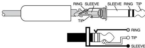
1/4" TRS Balanced Mono Wiring:
