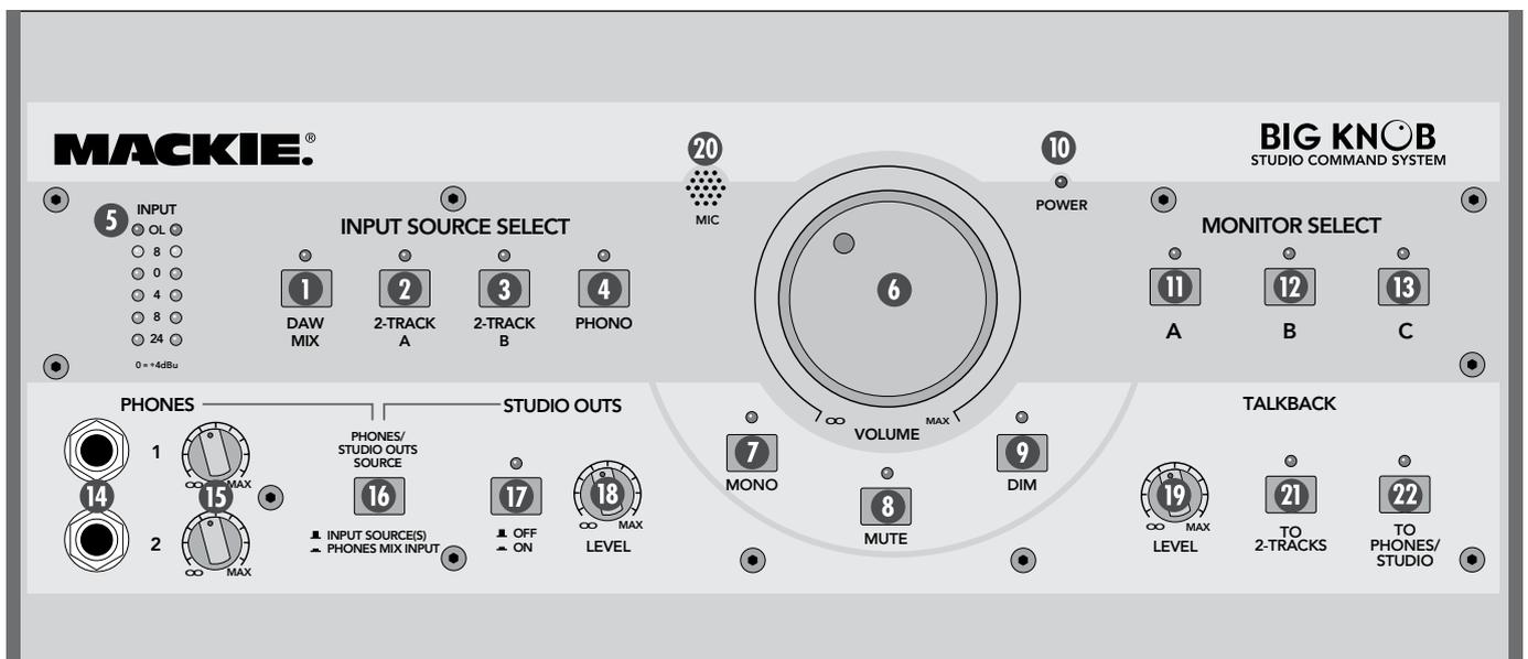
When the button is down (PHONES MIX INPUT), the STUDIO/PHONES outputs are fed the signal from the DAW PHONES MIX INPUT 35 jacks on the rear panel. In this position, the recording engineer listens to the “real” mix coming from the DAW (DAW MIX INPUT), but the talent can listen to an alternate and specialized mix coming from the DAW (DAW PHONES MIX INPUT).
