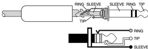
1/4" TRS Stereo Unbalanced Wiring:
