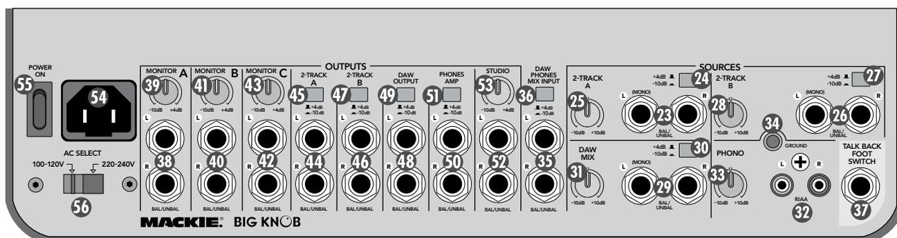
above the MONITOR A **38** output jacks is in the  $-10$  dB position (counterclockwise). If it is, turn the control up to the  $+4$  dB position and then turn up the Big Knob VOLUME control. Now it should get louder, faster.
